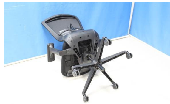
View 8 Conducted the back strength test – static on this chair according to applicant's requirement.
