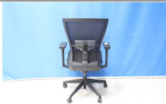
View 7 Conducted the back strength test – static on this chair according to applicant's requirement.
